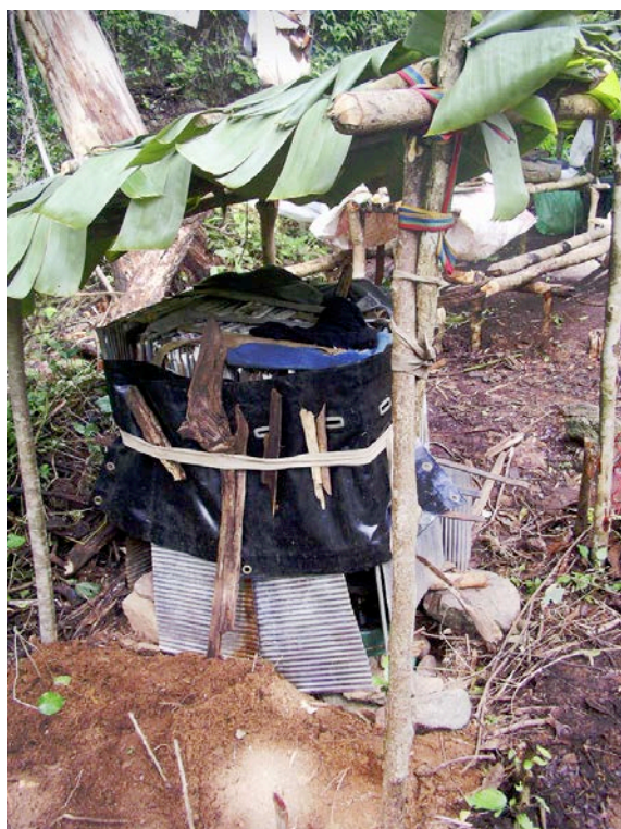
Field-drier for presses containing plant material from the Antsahabe Forest Massif (Loky-Manambato Protected Area, Madagascar, 2004). A gas cylinder is buried under the dryer. Operating 24 hours a day, it dries the botanical samples in a few days.
