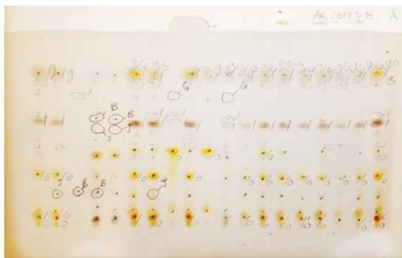
Lichenic substances revealed by thin-layer chromatography carried out in the Microscopy and chromatography laboratory.
